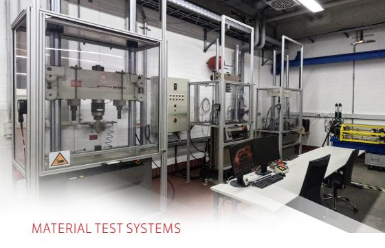
TGR-E has three MTS 810 uniaxial material test systems. The units use servo-hydraulic frames and can be customised to address a whole range of material testing demands. These test systems are suitable for large specimens and can accommodate various materials, including alloys and composites. TGR-E's range of material test systems includes MTS 318.10, 318.25 and 318.50 models.
