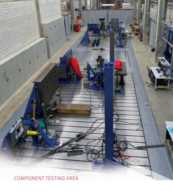
In this specific area of TGR-E's chassis testbench department, we offer various component durability and reliability tests. With our customizable and modular test equipment, we combine wide range of actuators and sensors for mechanical component tests.
