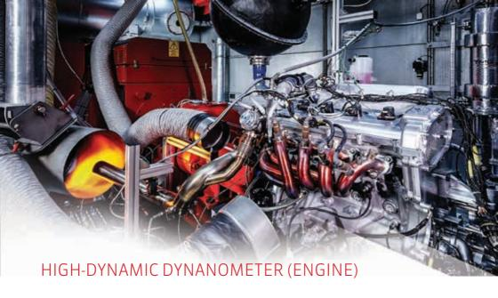
This high-dynamic engine dynamometer is designed for investigation of all engine-related aspects and allows extremely high performance engines to be tested to their full potential. Additionally, the inertia of the dyno's electric motor is equal to that of a race car wheel for greater accuracy.
