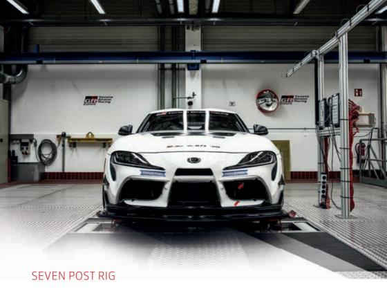
Our seven-post rig adapts to most vehicles and is a valuable development and proving tool for original equipment manufacturers and high-performance car developers. Our baseline configuration, featuring one frontal downforce actuator and two at the rear, is ideal for optimising the vertical dynamics of cars generating large amounts of downforce.
