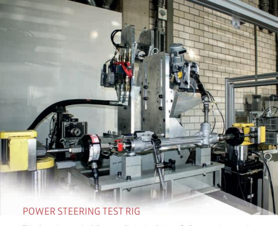
This dynamic test rig delivers realistic simulation of all suspension, turning and driving torque forces. A variety of different power steering solutions can be tested for durability and performance. For exceptional realism, simulated car or recorded track data can be used to test specific scenarios.
