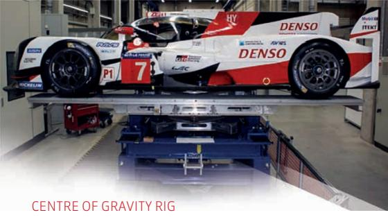
A specially-developed rig to determine, to a very precise level, the centre of gravity of a vehicle and the moment of inertia around the three main axes. Various complete cars can be mounted in exact road/track specification, up to a maximum weight of approximately 2,300kg.
