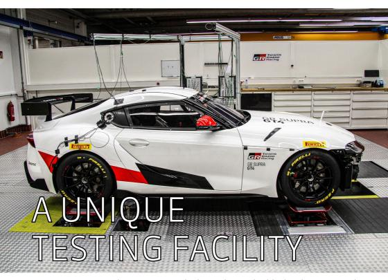
Our seven-post rig adapts to most vehicles and is a valuable development and proving tool for original equipment manufacturers and high-performance car developers. Our baseline configuration, featuring one frontal downforce actuator and two at the rear, is ideal for optimising the vertical dynamics of cars generating large amounts of downforce.
