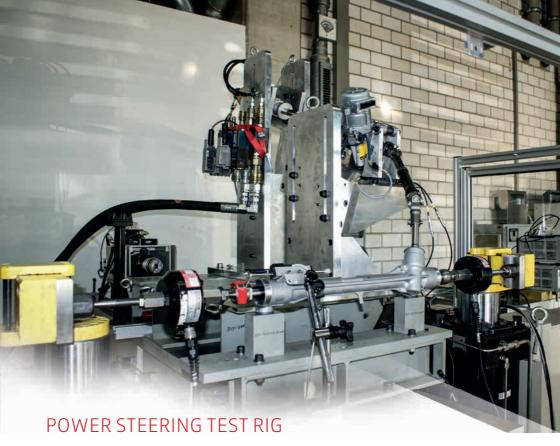
This dynamic test rig delivers realistic simulation of all suspension, turning and driving torque forces. A variety of different power steering solutions can be tested for durability and performance. For exceptional realism, simulated car or recorded track data can be used to test specific scenarios.
