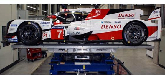
A specially-developed rig to determine, to a very precise level, the centre of gravity of a vehicle and the moment of inertia around the three main axes. Various complete cars can be mounted in exact road/track specification, up to a maximum weight of approximately 2,300kg.
