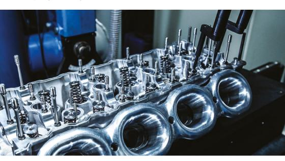
This rig allows precise and in-depth port development to deliver optimal performance by analysing air flow through the intake and exhaust ports of the cylinder head. Particle Image Velecimetry is also offered for unbeatable accuracy and analysis. The rig features suction and blowing stations; both offer flow measurement possibilities while suction mode additionally allows swirl and tumble analysis.
