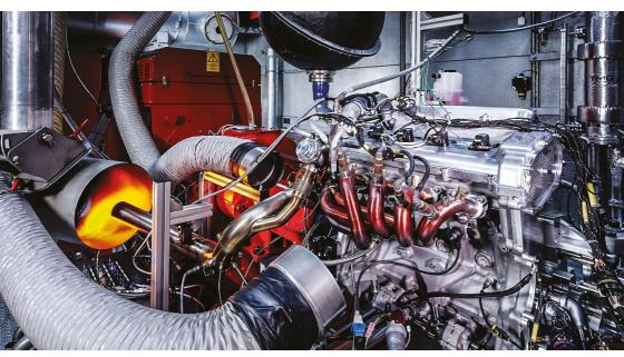
This high-dynamic engine dynamometer is designed for investigation of all engine-related aspects and allows extremely high performance engines to be tested to their full potential. For hardware-in-the-loop testing, specific car or wheel models can be implemented using Matlab Simulink on dSPACE HIL. Additionally, the inertia of the dyno's electric motor is equal to that of a race car wheel for greater accuracy.
