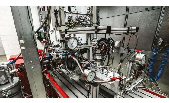
The component rigis a bespoke unit which allows ancilliary engine components to be tested in isolation. It can be customised for various purposes and part sizes.
