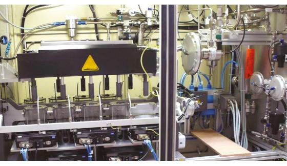
Designed to optimise fuel spray for performance and efficiency, this specialist system can also condition the fuel temperature and pressure. This versatile rig features separate systems for fuel pumps, injector rails and single injectors. Malvern laser system and high-speed camera analysis is also available on these rigs. Customer ECUs and injector power units can be implemented
