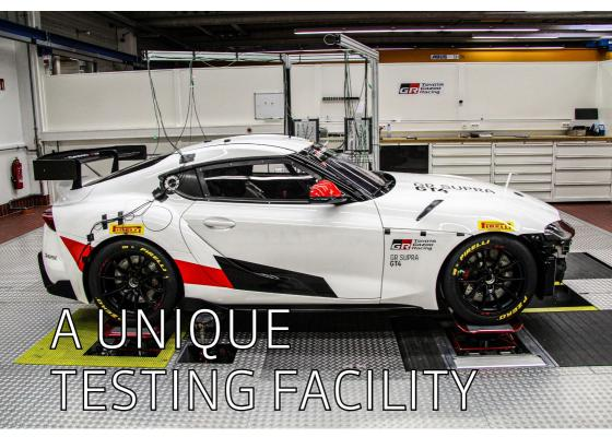
Our seven-post rig adapts to most vehicles and is a valuable development and proving tool for original equipment manufacturers and high-performance car developers. Our baseline configuration, featuring one frontal downforce actuator and two at the rear, is ideal for optimising the vertical dynamics of cars generating large amounts of downforce.
